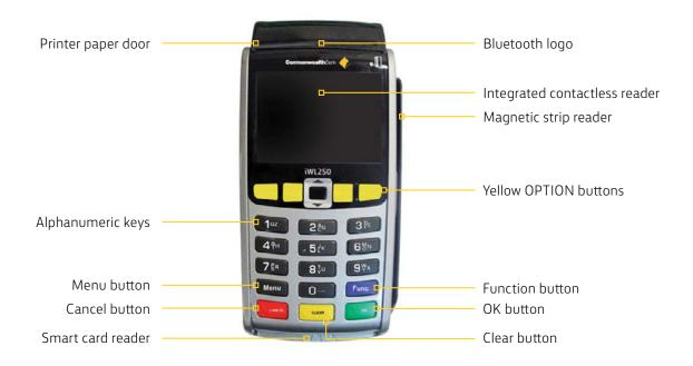
**Note:** The first three yellow option buttons will be used as the **Cheque**, **Savings** and **Credit** keys. The fourth soft key will not be used. During Idle state, only the [Menu] and [Func] buttons are operable. Pressing either button will open the Main Functions Menu.
