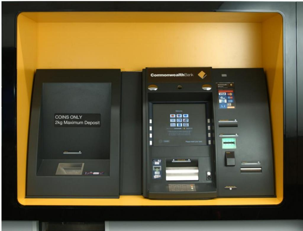
Figure 6. The coin compartment is on the left side of ATMs.
